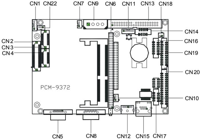
*Figure 2.2: Connectors (component side)*
