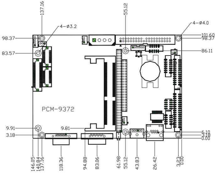
*Figure 1.1: Board layout: dimensions*
