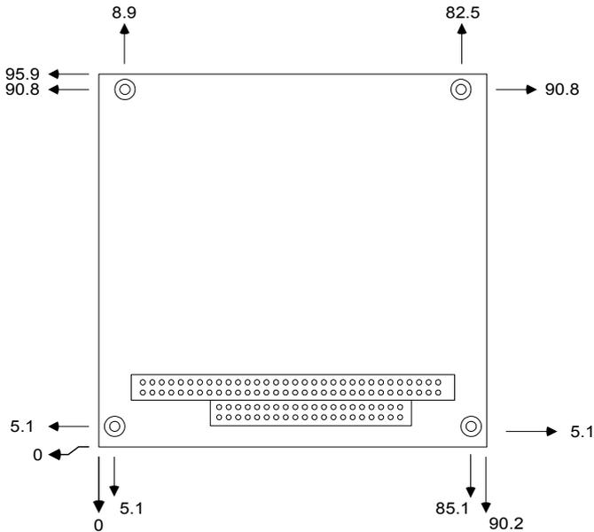
**Figure B.2: PC/104 module dimensions (mm) ( $\pm 0.1$ )**
