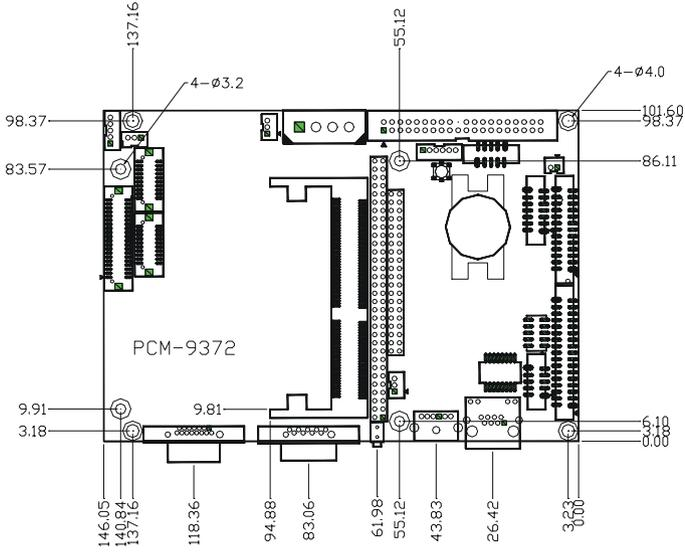
**Figure F.1: PCM-9372 Mechanical Drawing (Component Side)**
