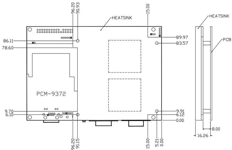
**Figure F.2: PCM-9372 Mechanical Drawing (Solder Side)**
